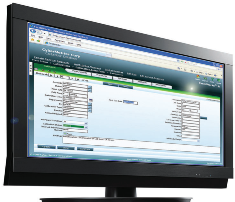
Shown is an example of a Web-based calibration management module that is part of a larger enterprise asset management system. Source: CyberMetrics
